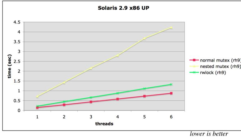
Solaris is impressively stable as the number of threads increase during the test. Since APR's normal mutexes and rwlocks are implemented on Solaris as a very thin layer above the operating system, this test demonstrates Solaris' impressive ability to scale with both rwlocks and mutexes. The severe penalty for using APR's nested mutexes is very evident in this graph.
