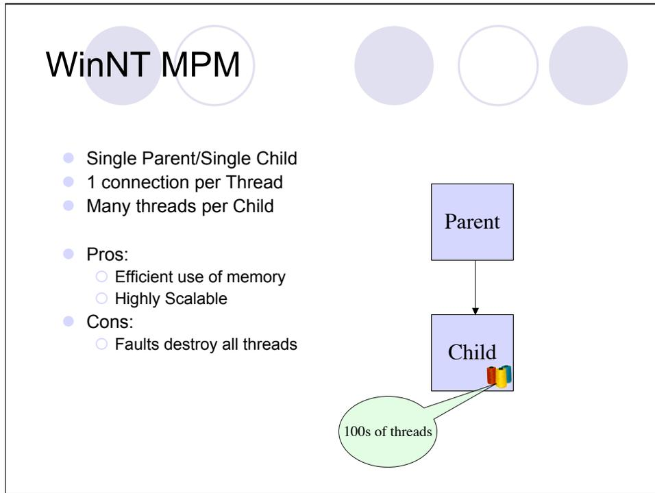
The WinNT MPM is specifically customized for the Windows platform. It has one parent and one child, with the single child having many hundreds of concurrent threads. Each thread handles a separate request connection.
