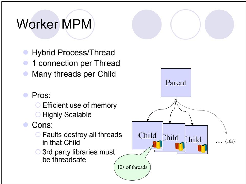
The worker MPM is the new hybrid multiprocess/multithreaded model specifically targeted by Apache 2.0. This MPM trades a small amount of fault isolation for massive scalability (especially in terms of memory consumption). It performs on par or slightly under par with a lightly loaded prefork MPM server, but is able to handle many more concurrent connections without significant memory consumption.
