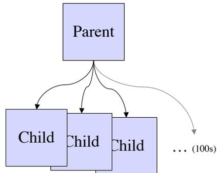
Available on Unix. This MPM matches the model used since NCSA and through Apache up to Apache 1.3. In general it tends to perform well on uniprocessor machines, and is highly robust. The prefork MPM is not well suited for high-traffic, highly concurrent systems. Although the prefork MPM processes many hundreds of simultaneous connections without problem, systems are usually limited by the amount of memory consumed.
